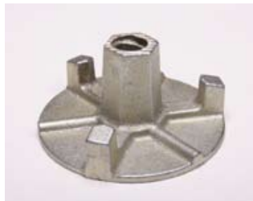
100mm Dywidag Tie Nut Used to secure Working Platform Brackets, Walers & Dywidag Pin.
