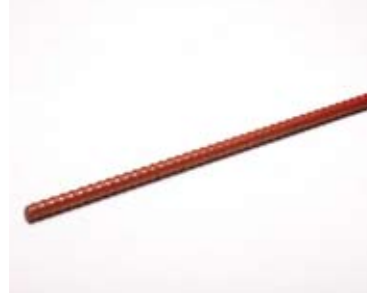
Dywidag Rod Used in place of the flat wall ties when wall thickness exceed 450mm.
