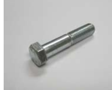
M16 x 80mm Bolt (Kicker Bolt) Used to anchor the Kicker in position after concreting is finished (reusable item).
