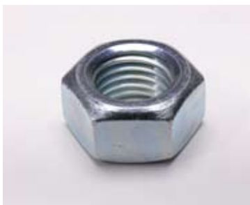
M16 Nut Used in conjunction on the securing the M16 x 80mm Kicker Bolt (Consumable Item) Also used to assist the securing of the M16 x 30 Bolt for permanent fixings.
