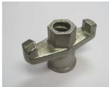
Dywidag Wing Nut Used to secure the Vertical Soldier that controls alignment at slab level.
